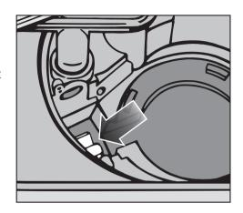
The drain pump is located beneath the non-return valve (arrow).
